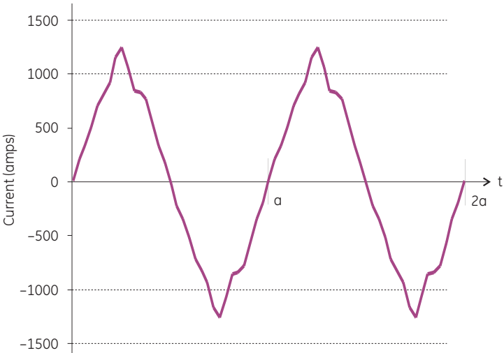
FIGURE 2-11: Distorted Current Waveform
